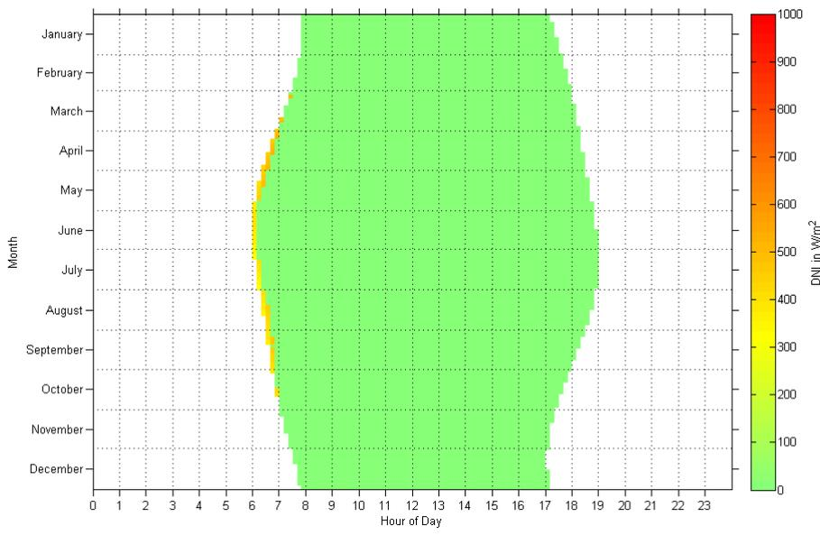
**Figure 8: Shading Impact on BirdDNI for Sun Elevations >5°**
