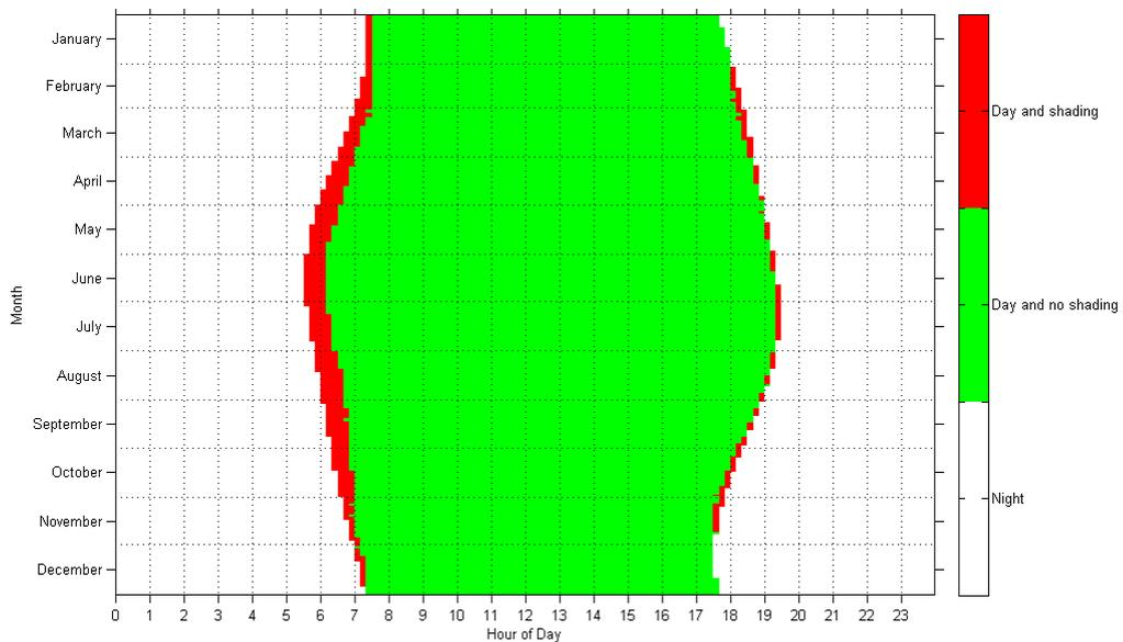
**Figure 6: Shading Table for Sun Elevations >0°**
