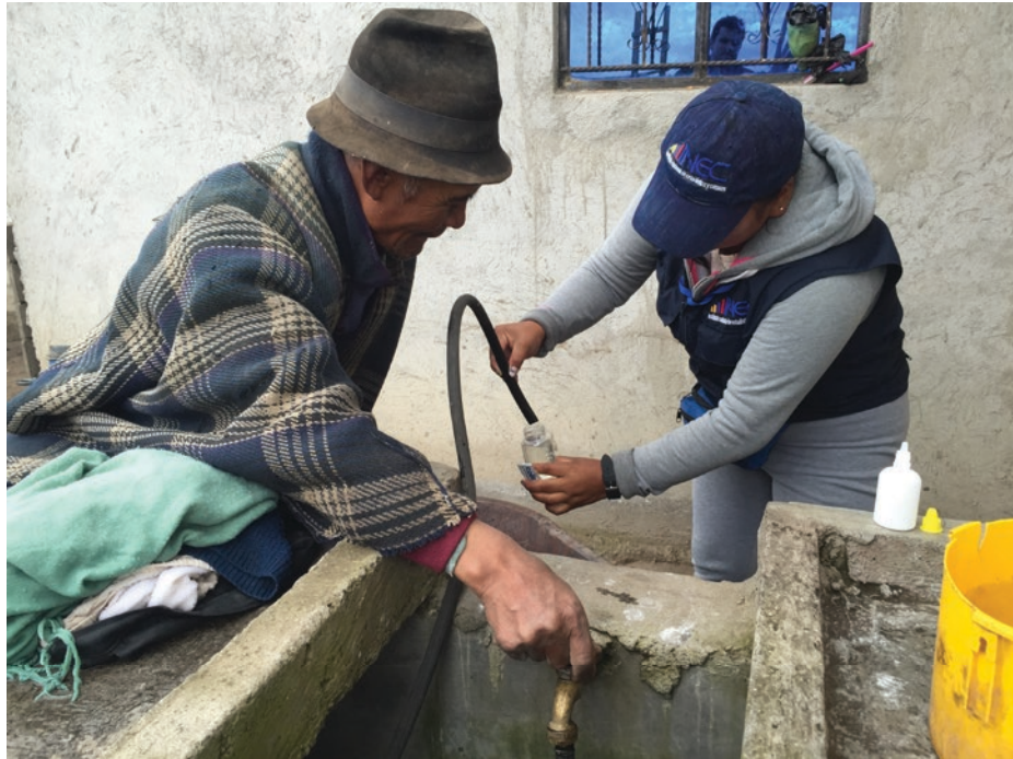
Photo 3.1: Enumerator Taking a Water Sample for E.coli Presence Test
