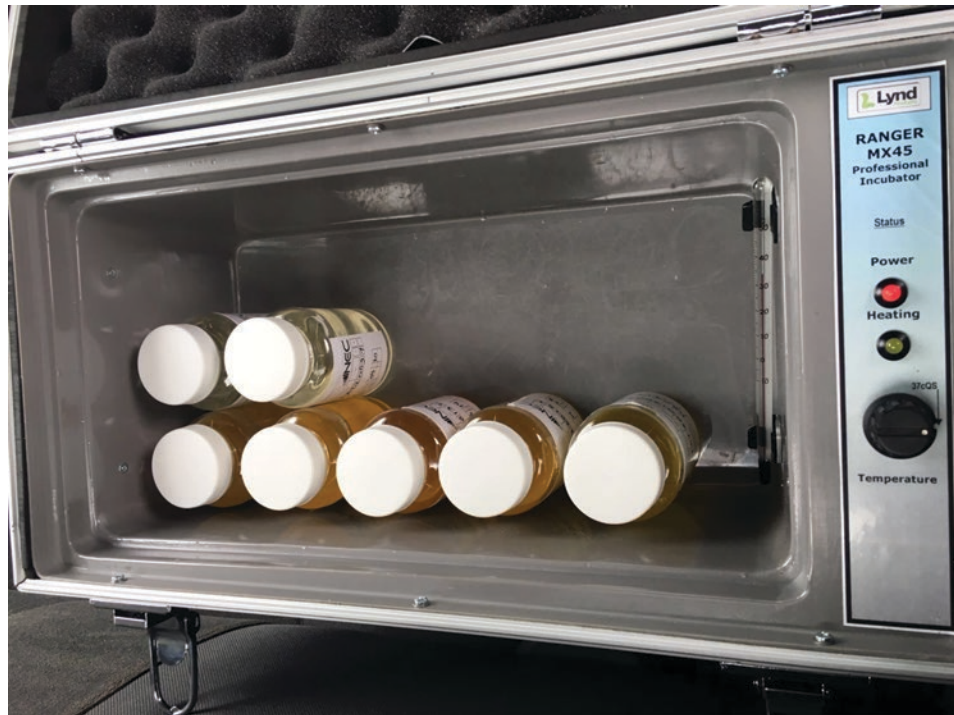
Photo 3.2: Incubator Holding Water Samples for Testing
