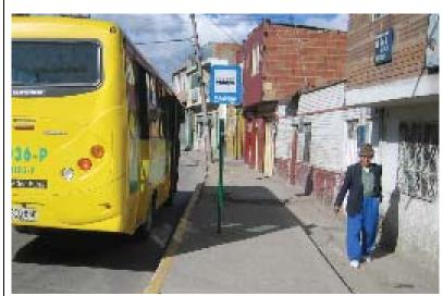
The photo at left shows an improved bus stop on а TransMilenio feeder route on the outskirts of Bogotá, Colombia. The all-weather concrete pad, vellow curb. and route sign (with pictograph in contrasting colors) enhance the use of this stop.
