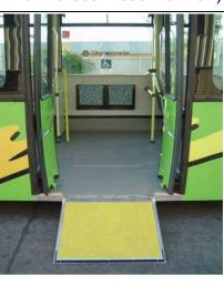
The photo at left, courtesy of Transantiago, illustrates the use of a simple manually operated ramp to provide access to a low-floor bus in Chile. See COST 322, under Resources, for more information on low-floor buses, or contact Transantiago.
