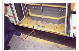
Raised bus stops can reduce the the distance to first step. provided that other vehicles do not block the stop and drivers are trained and monitored to stop adjacent to the stop. The photo at top shows a currently used feeder bus in a Colombian city with a first step that is especially high when boarded from ground level. The photo at bottom shows the impact of a lower first step and proper alignment with a raised bus stop, providing a far more accessible step. (Each mark on the rulers = 50 mm.)
