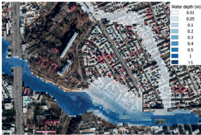
Flooding caused by simulated dam break. Increasing water depth shown in darker blue
