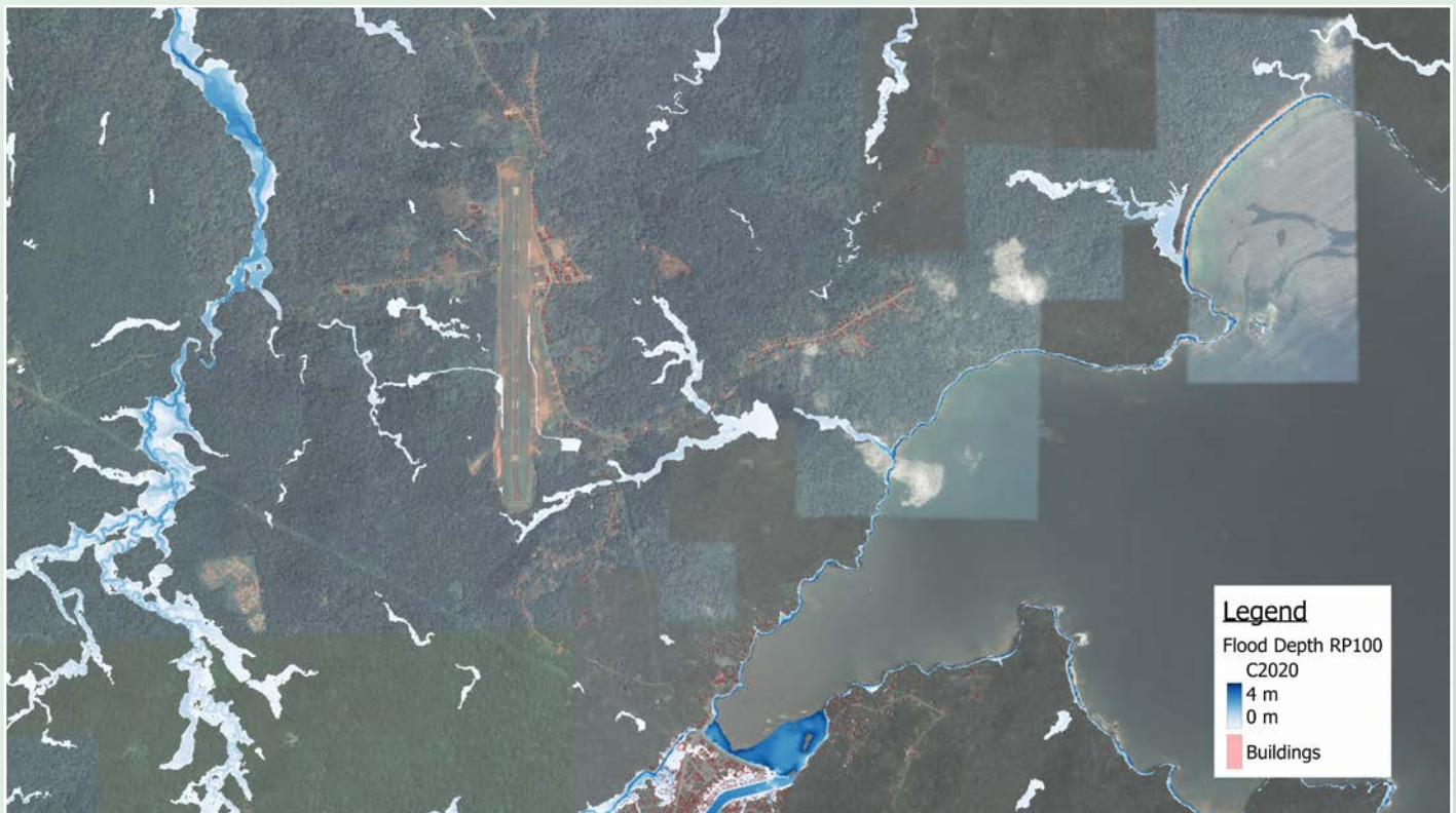
Airport of Príncipe and access roads (flood hazard RP100, present climate).
