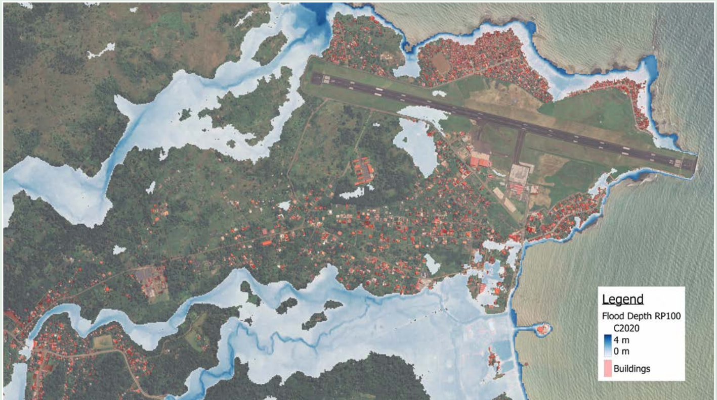
Airport of São Tomé and access roads (flood hazard RP100, present climate).
