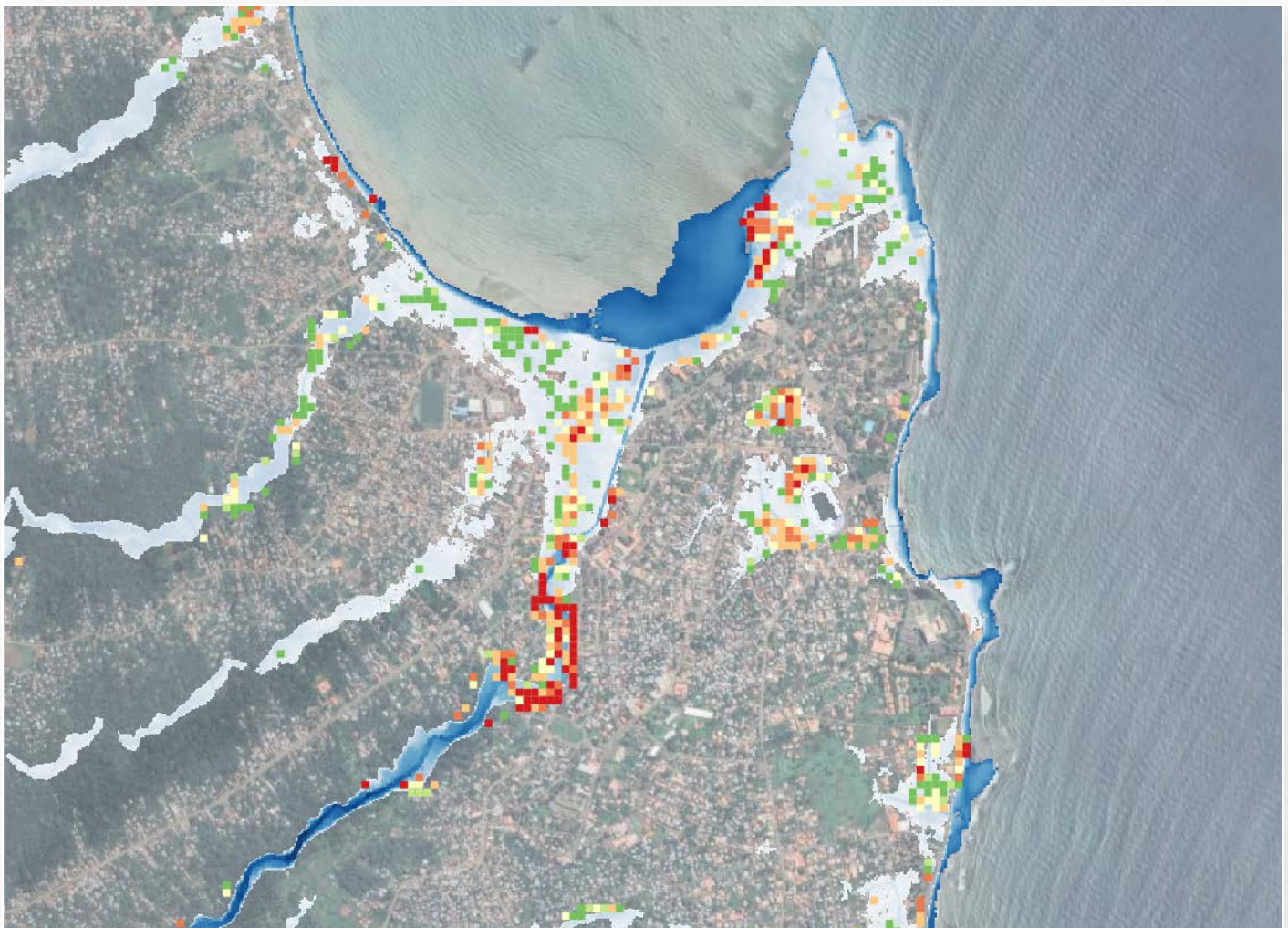
Fine-resolution flood risk results for the city of São Tomé using the cell-based risk assessment approach as the basis for the tabular results per (modified) subdistrict.
