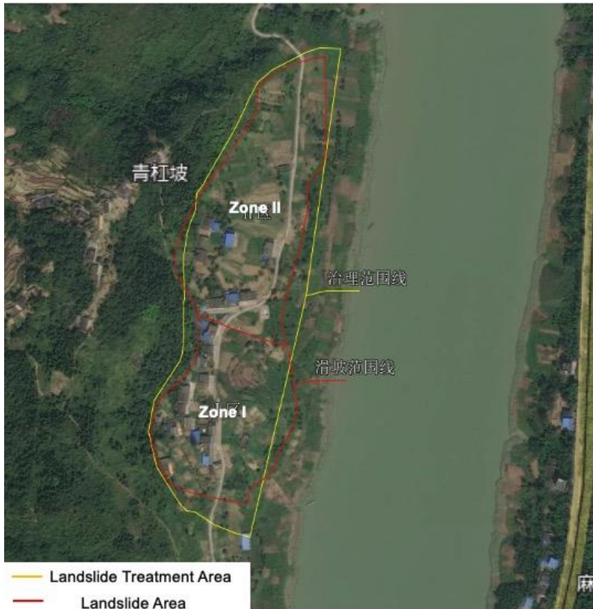
Figure 2 Guihuabang Landslide Area and Treatment Area
