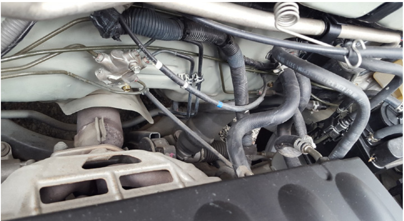
Image 1.1. Tampered Car in an East African Country, with Catalytic Converter and Antilock Brake System Removed
