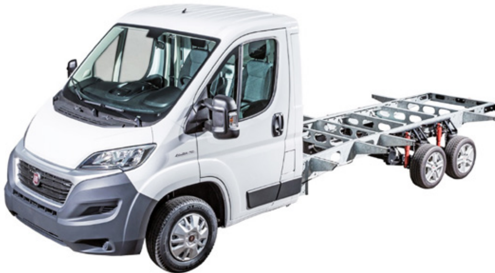
Image 4.2. Example of Single-Unit Truck Cab and Chassis (Fiat Ducato from AL-KO)
