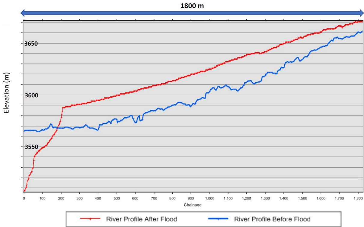
7a) longitudinal section showing the river profile before and after the flood
