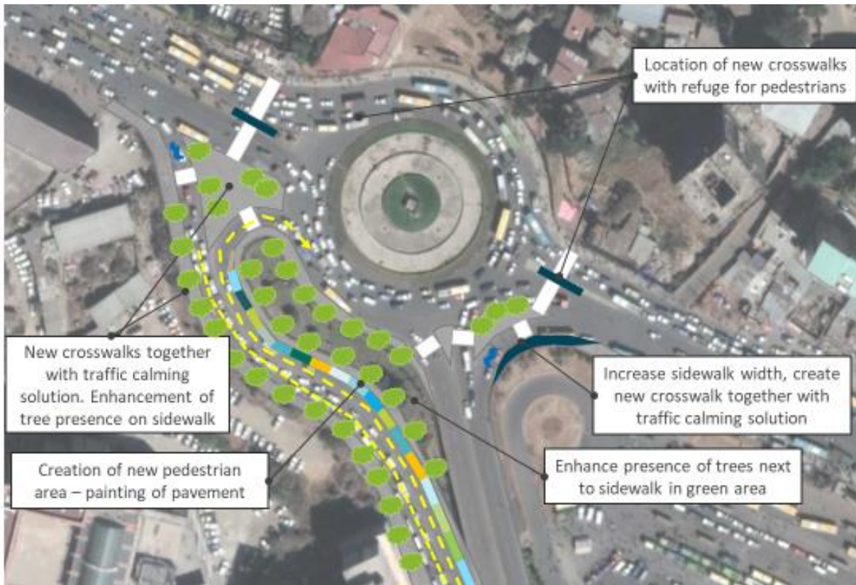
Figure 41. Conceptual proposal for redesigning the Wal-Argi square area and enhancing the connection between Megenagna Station and Wal-Argi square.
