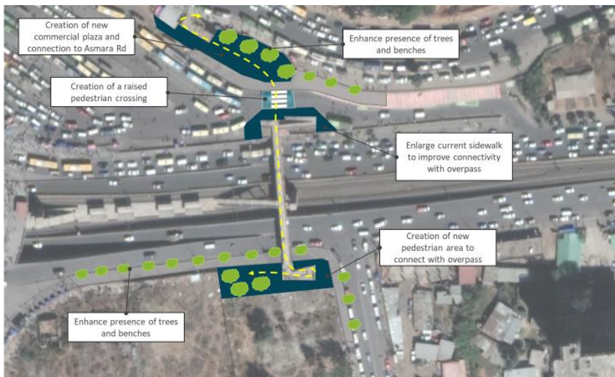
Figure 43. Conceptual proposal for improving connectivity between the LRT station and the nearby urban area and bus station.
