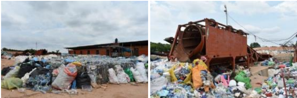
Figure 17 The Waste Retailer at the Landfill in Kaysone Phomvihane with a Rotary Drum Screen
