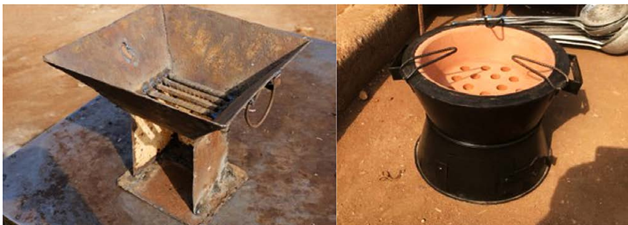
Photo 17. Traditional coal pot and improved Gyapa charcoal stove, Tamale, Northern Region
