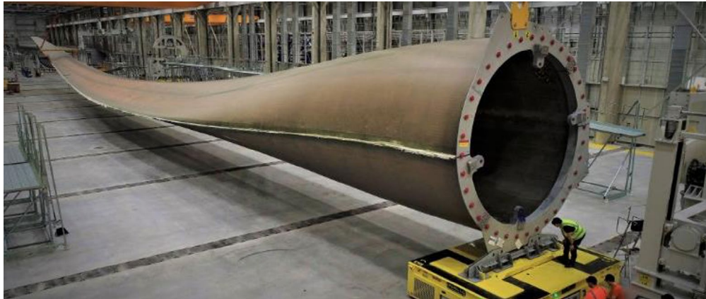
FIGURE 12.4 LM WINDPOWER'S 107 M LONG BLADE IS THE LONGEST DEPLOYED TO DATE [87].
