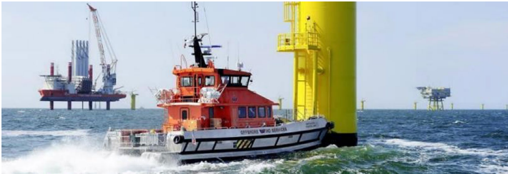
FIGURE 12.10 CREW TRANSFER VESSEL AT A WTG (SOURCE: COWI).
