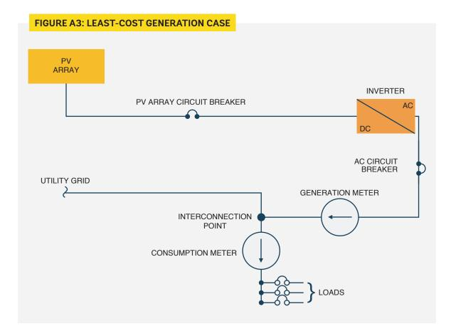
is installed on or nearby a building (which serves as a host to the PV system), the PV system is not a part of the building's electrical system. There is no direct electrical connection between the PV system and any building infrastructure other than through the grid. The configuration requires two meters, one for the electricity fed from PV into the grid and the other on the customer side measuring the customer's electricity use.
