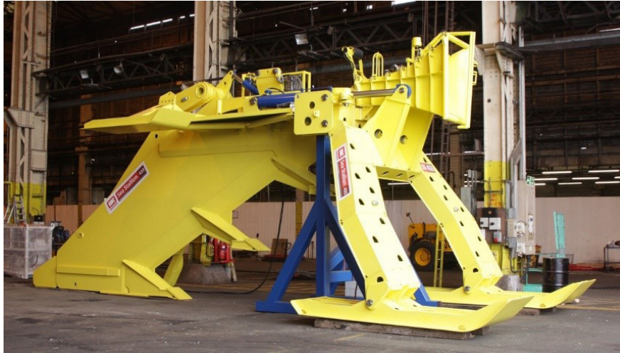
FIGURE C7.4 EXAMPLE CABLE PLOUGH
