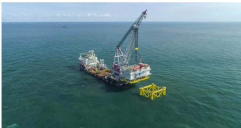
FIGURE C7.2 EXAMPLE SUBSTATION INSTALLATION VESSEL
