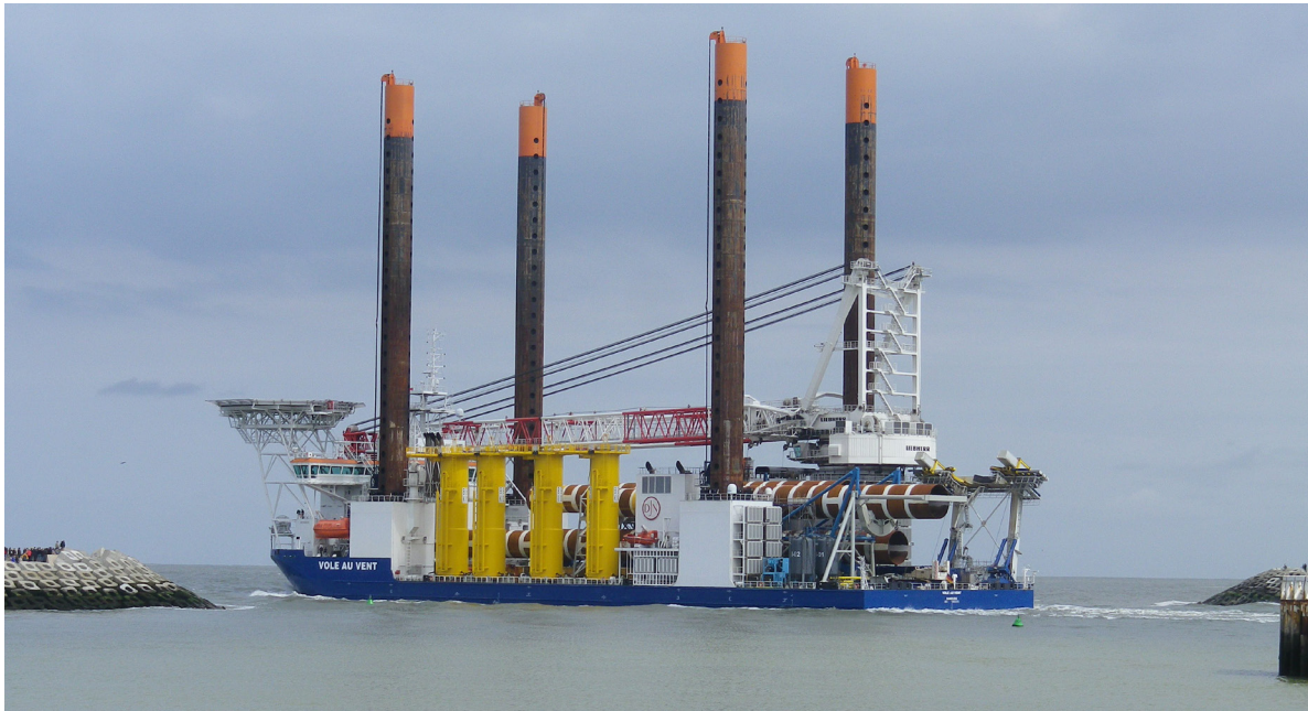
FIGURE C7.1 EXAMPLE MONOPILE FOUNDATION INSTALLATION VESSEL
