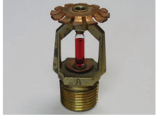
Figure 35. Exemplar sprinkler head
