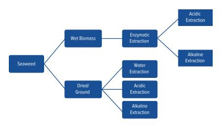
FIGURE 8: Biostimulant processing flow
