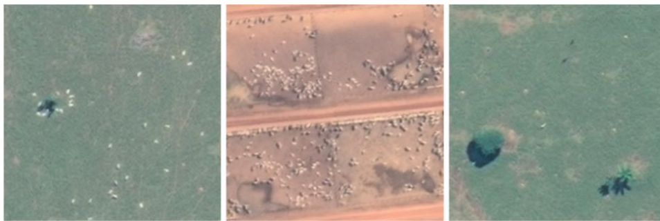
Figure A4. Counting cows from Brazilian ranches through satellite images with 40cm or better resolution (after pansharpening), and with less than 20% cloud coverage. Left: Typical image with cattle. Center left: Crowded ranch.. Center right: There is likely a white cow in the middle, while the rest of the white blobs appear due to lack of vegetation. Image ©2020 Maxar Technologies. From: Laradji et al. (2020). Counting Cows: Tracking Illegal Cattle Ranching From High-Resolution Satellite Imagery. arXiv preprint arXiv:2011.07369.
