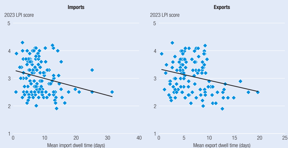
Figure 3.4 Import and export dwell time of containers, May–October 2022, versus 2023 LPI score, by country
