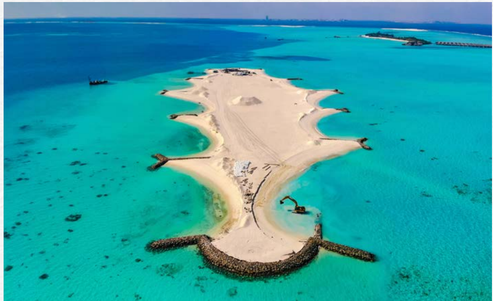
Photo Description: An Island being developed for inhabitation in the Maldives. © Juergen Rudolf
