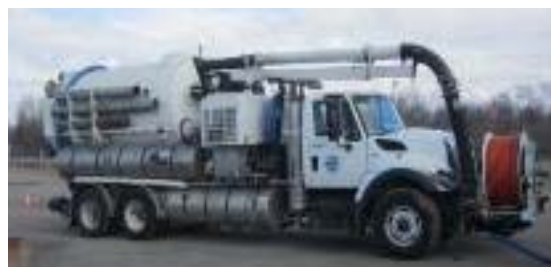
Photo 3.5 Insulated Vacuum Truck
