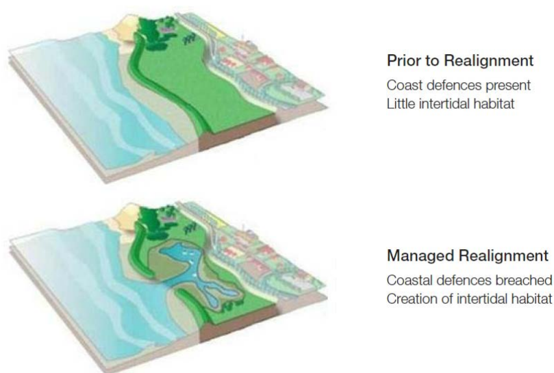
Figure 3-3: Schematic of the concept behind the managed realignment option (Linham and Nicholls, 2010)
