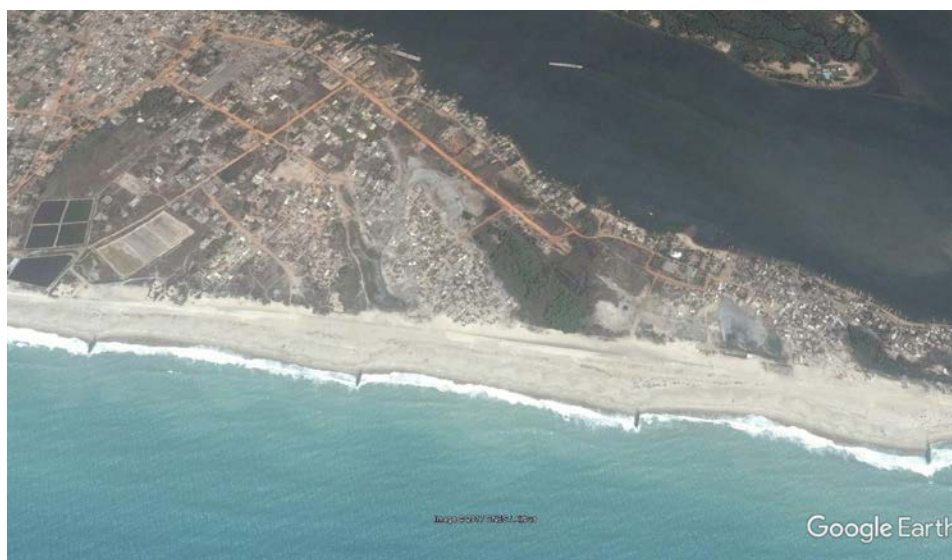
Figure 3-2: Groynes as stabilisation measure for beach nourishment and dune building - Ada, Ghana
