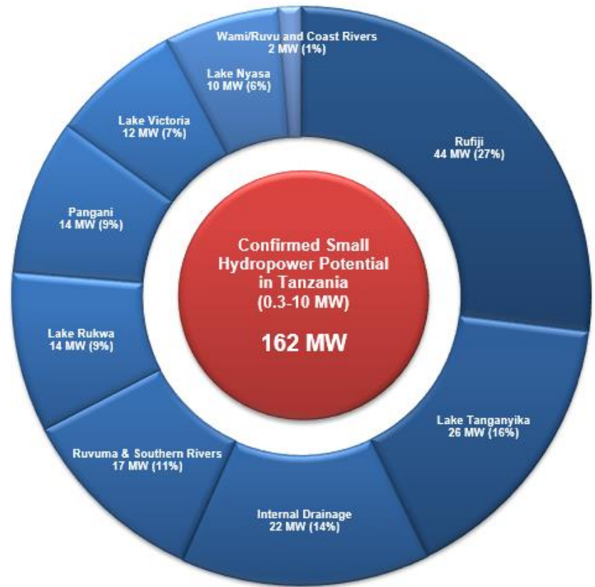
Figure 14. Small hydropower potential (0.3-10 MW) confirmed by site visits: breakdown by water basin.
