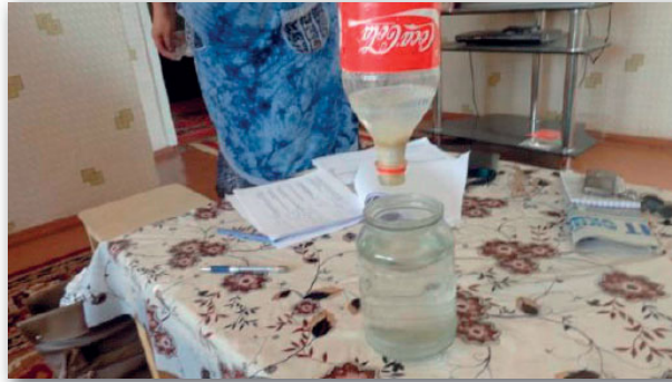
Photo 7. Water filtration using cotton wool in the neck of the bottle, Tashkent
