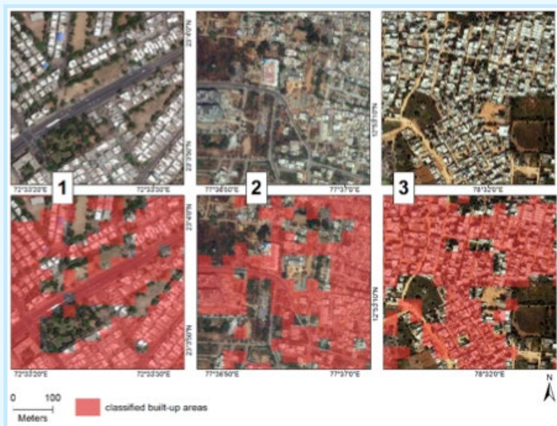
Figure 2: Classification of built-up areas (visualized in red) compared to raw satellite images in three regions in India (Classifier: Random Forest with 10 trees; Input: Landsat 8).
