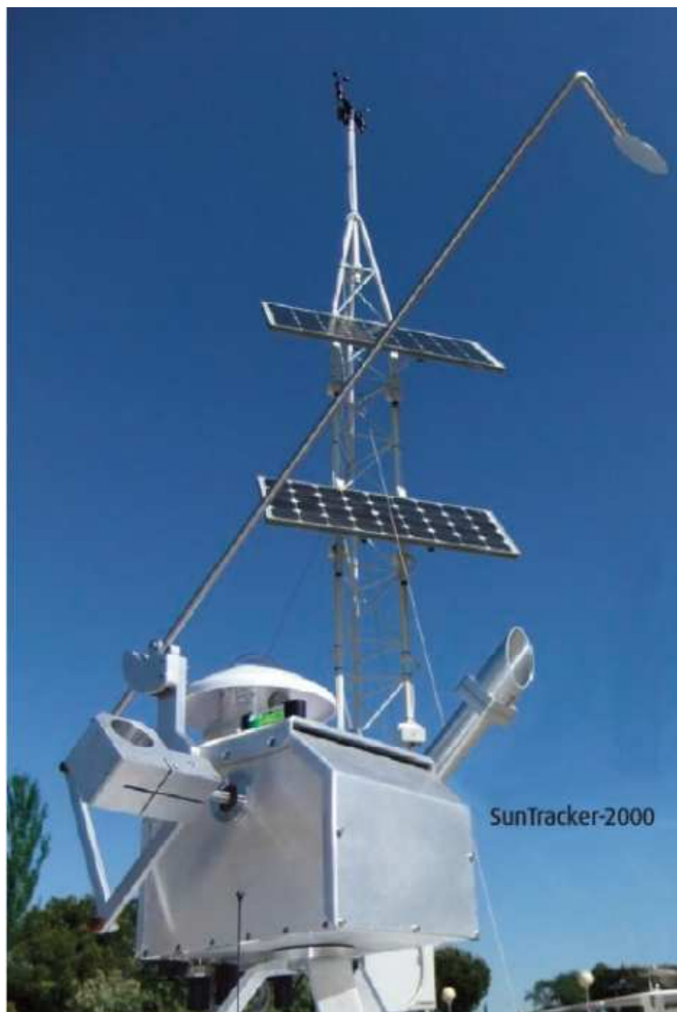
Fig 28 Tier 1 station: Suntracker and meteo tower.
