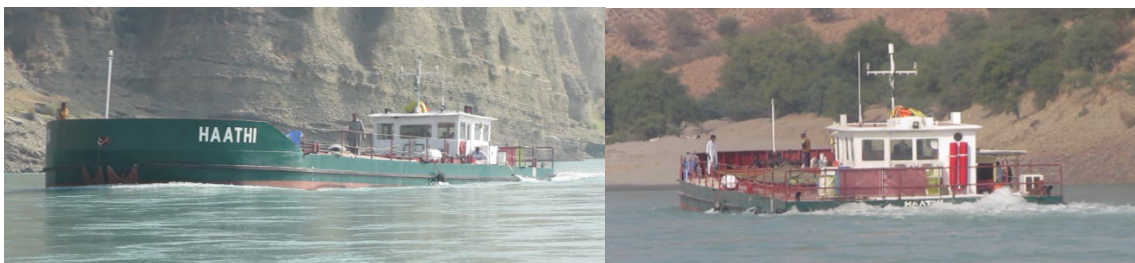
Figure 14: Vessel "Haathi" (35m x 9.5m x 1.5m) fabricated by IWTDC sailing north of Makhad
