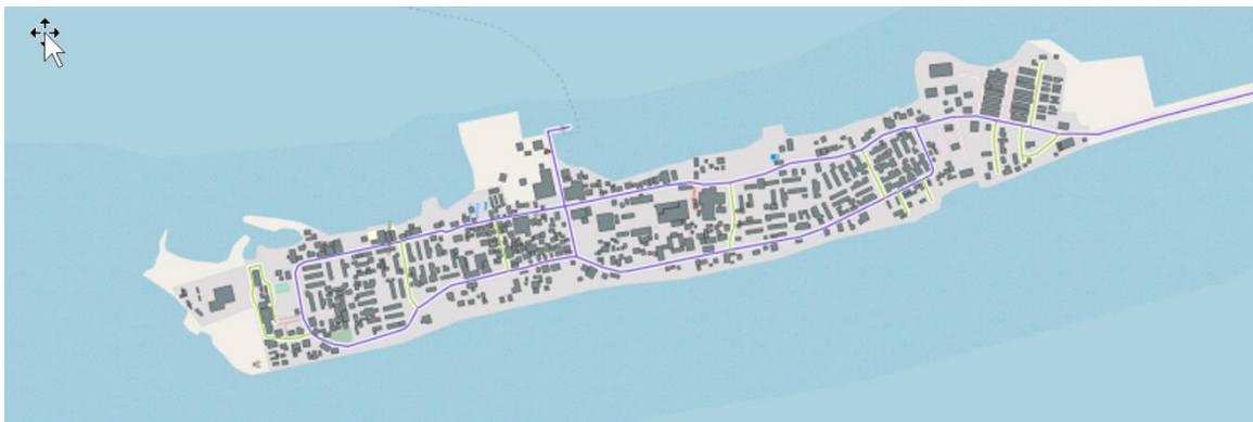
Figure 2 - Ebeye showing the expected main fiber path
