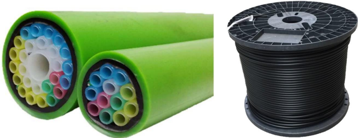
Figure 25 - Hexatronic Tight Protected Microduct products as examples. .On the left are the Ribbonet products with the larger duct having 26 5/3.5mm ducts for individual premises and a single 12/10mm duct for feeder or core fiber. The overall duct is 38mm in diameter resulting in a low impact installation compared to traditional ducting. The drum on the right is a 500m drum of
