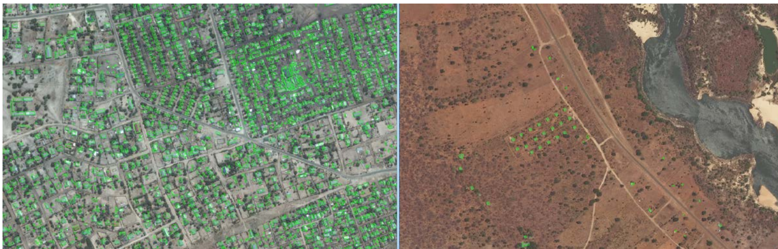
Satellite imagery and machine learning used to detect rooftops, designated by the green outlines, in Djibouti. Left: An urban area in Djibouti. Right: A rural area in Djibouti.
