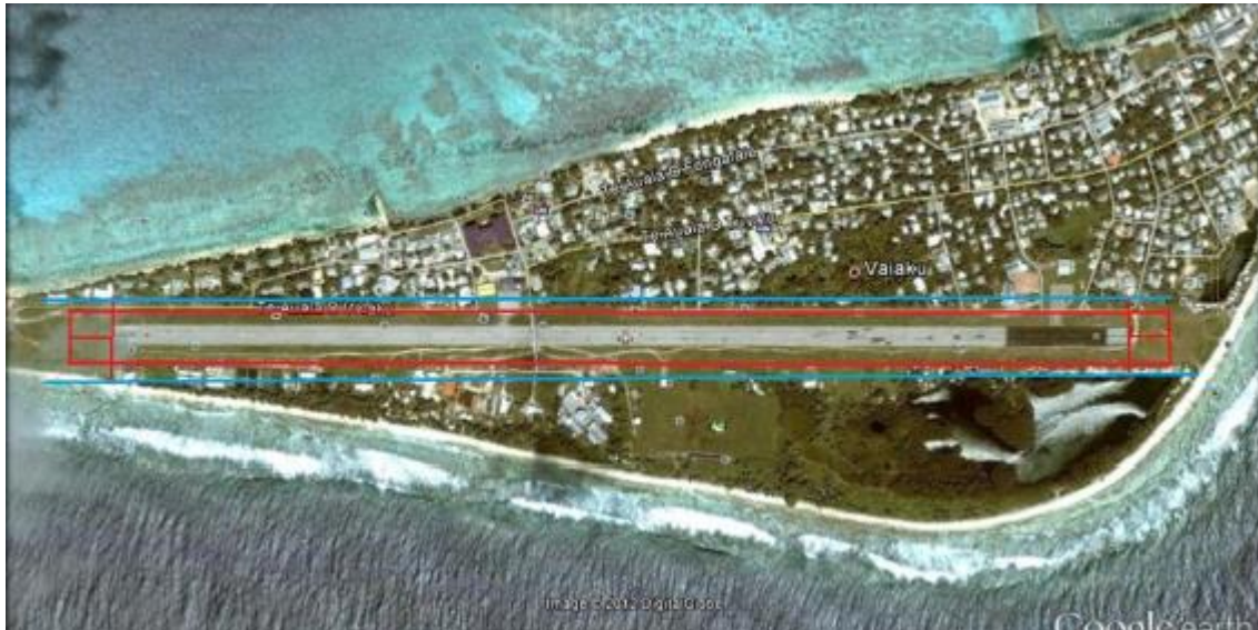
Figure 1: Funafuti Airport with the existing 80m runway strip and transitional OLS protection limit for structures of 4m shown as blue line (from: (GOT, 2013b)). Some of the road network is also visible in this map.
