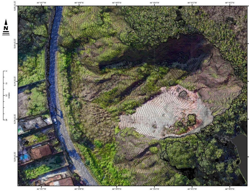
FIGURE 3.7 MAP GENERATED IN A GIS ENVIRONMENT, CONTAINING THE IMAGE, MDS, AND ISOLINES (AERO PHOTOGRAMMETRIC SURVEY DATA USING AN UAV)
