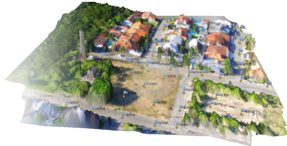
FIGURE 3.3 GROUND CONTROL POINTS SURVEYED WITH GPS L1, L2
