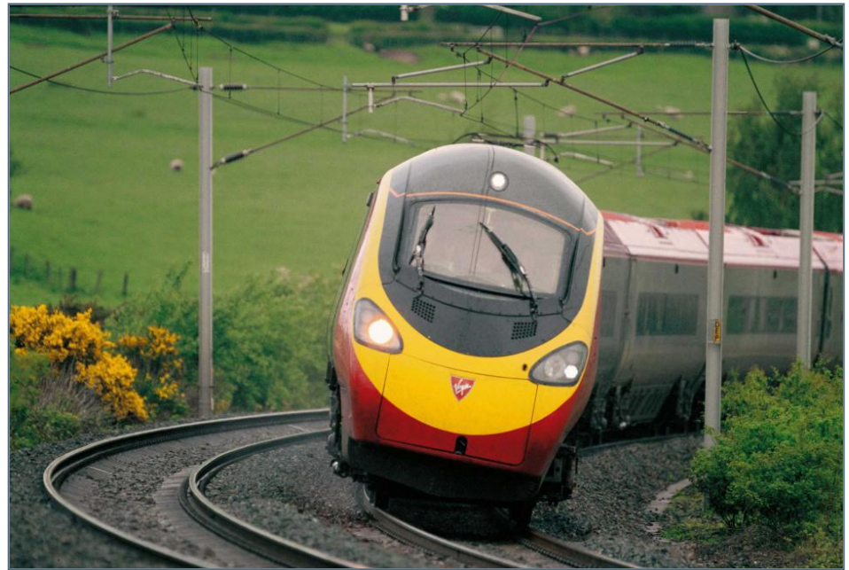
Pendolino using tilting technology (Source: Virgin website)
