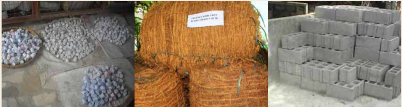
The Integrated Solid Waste Management Facility at Teresa, Philippines produces multiple products from recycled waste, including: paper charcoal (left), coconut husk netting (middle), and hollow concrete bricks filled with shredded plastic (right). Photo: Teresa Municipal Environment and Natural Resources Office.
