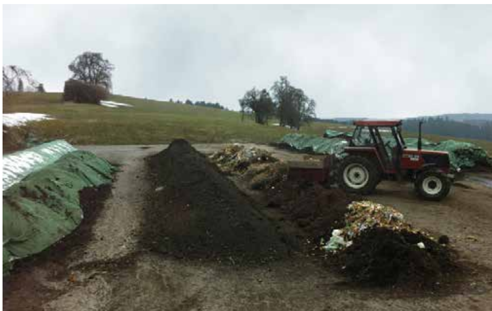
Fresh organic waste is added to windrows at an Austrian farm composting facility. Photo credit: 100-First Zero Waste & Organic Cycle Organisation
