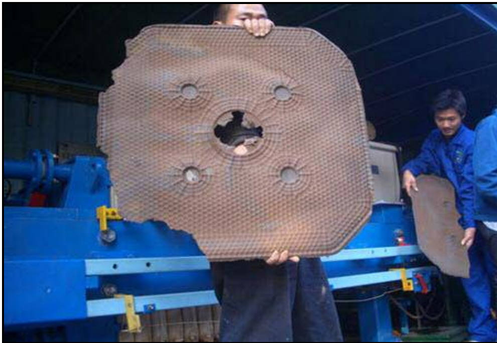
Figure 2.4-4 Sludge Cake after Advanced Dewatering
