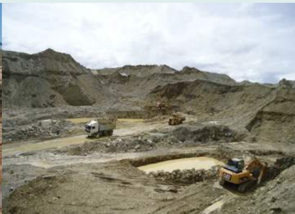
Semi-mechanized small-scale surface mining in Bolivia. Photo credit: Manuel Salinas
