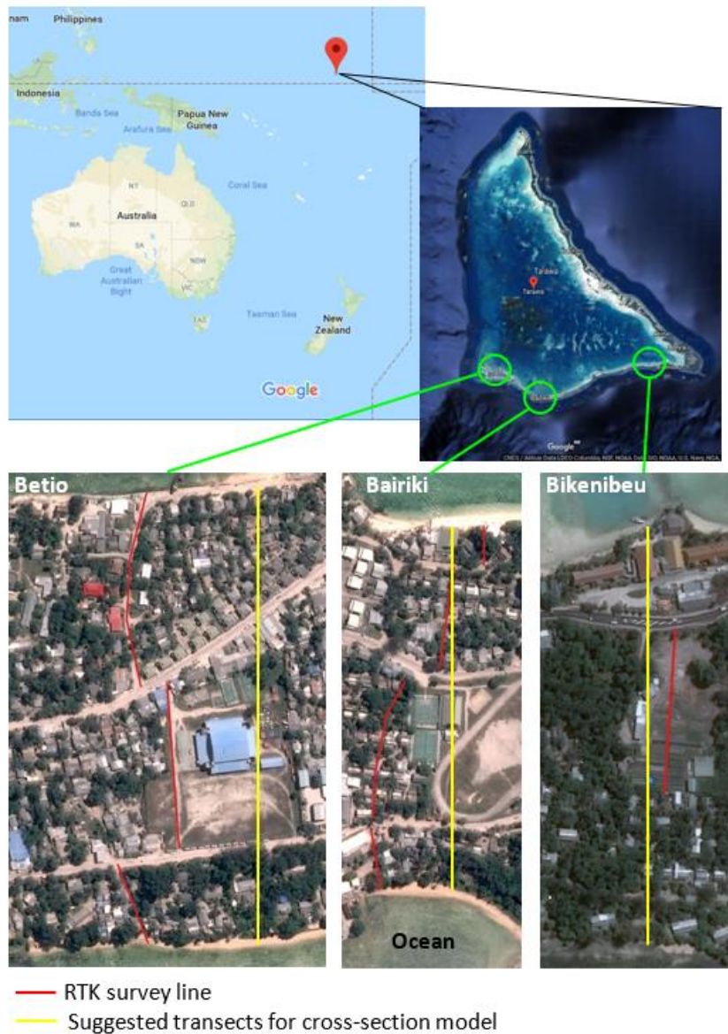
Figure 3. The location of RTK (real-time kinematic) survey lines and transects for cross-sectional models.
