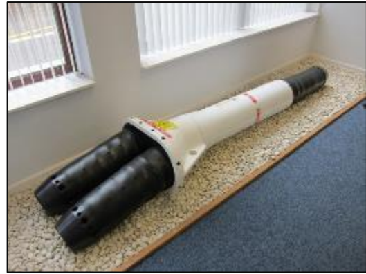
Figure 26: Example of a Branching Unit
