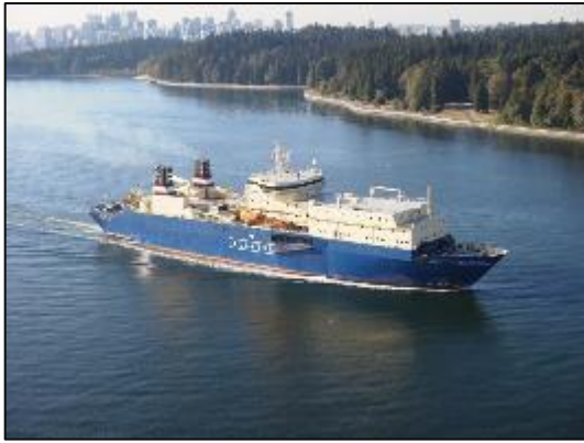
Figure 25: Typical cable laying vessel
