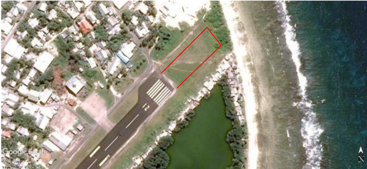
Figure 9: Approximate boundary of Funafuti International Airport runway end safety area (RESA) for runway end 21
