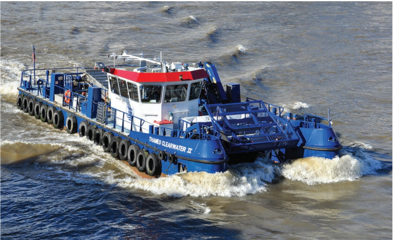
PHOTO 3.6. Trash Skimmer Boat That Removes Waste from Waterways
