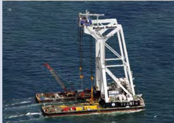
FIGURE B1.7: SPECIALIST INSTALLATION VESSEL: THE SVANEN
