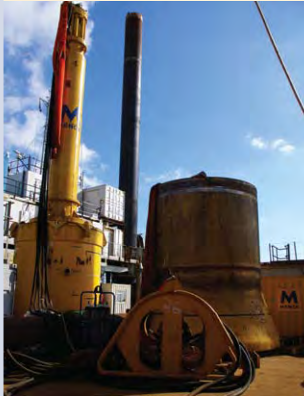
FIGURE B1.10: PILING HAMMER (LEFT) AND ANVIL/ADAPTOR PIECE (RIGHT)
