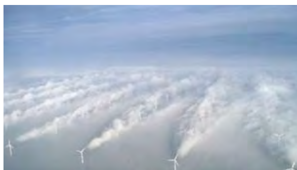
FIGURE A-1: ILLUSTRATION OF THE WAKE EFFECT
