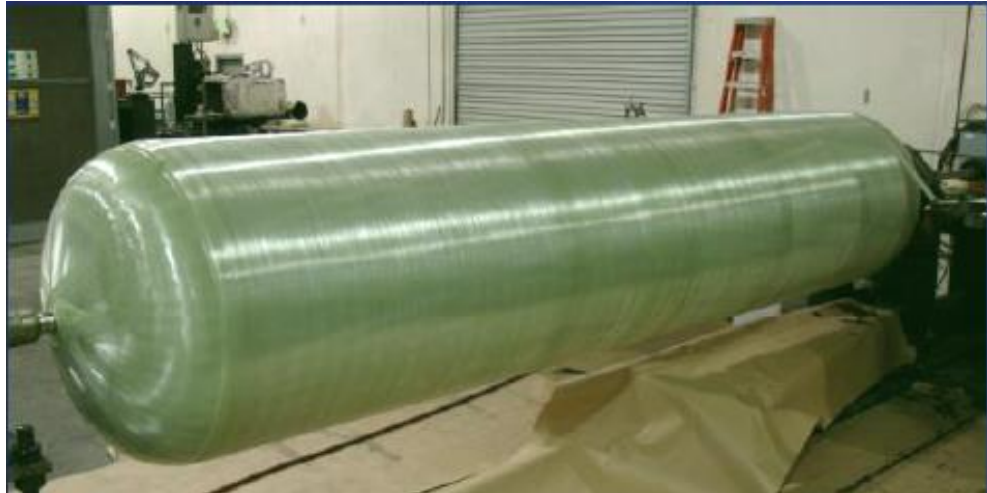
Figure 31 Prototype 1-Meter Diameter Pressure Vessel (Courtesy TOG Inc.)
