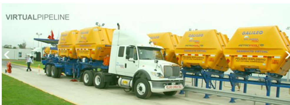
Figure 43 PAD platforms and MAT® gas storage modules (Courtesy Galileo)
