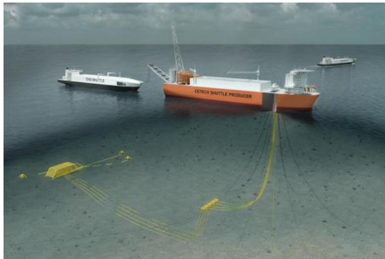
Figure 6 Floating Production Storage and Offloading (FPSO) with offloading to dedicated shuttle tankers (Courtesy of CETech)
