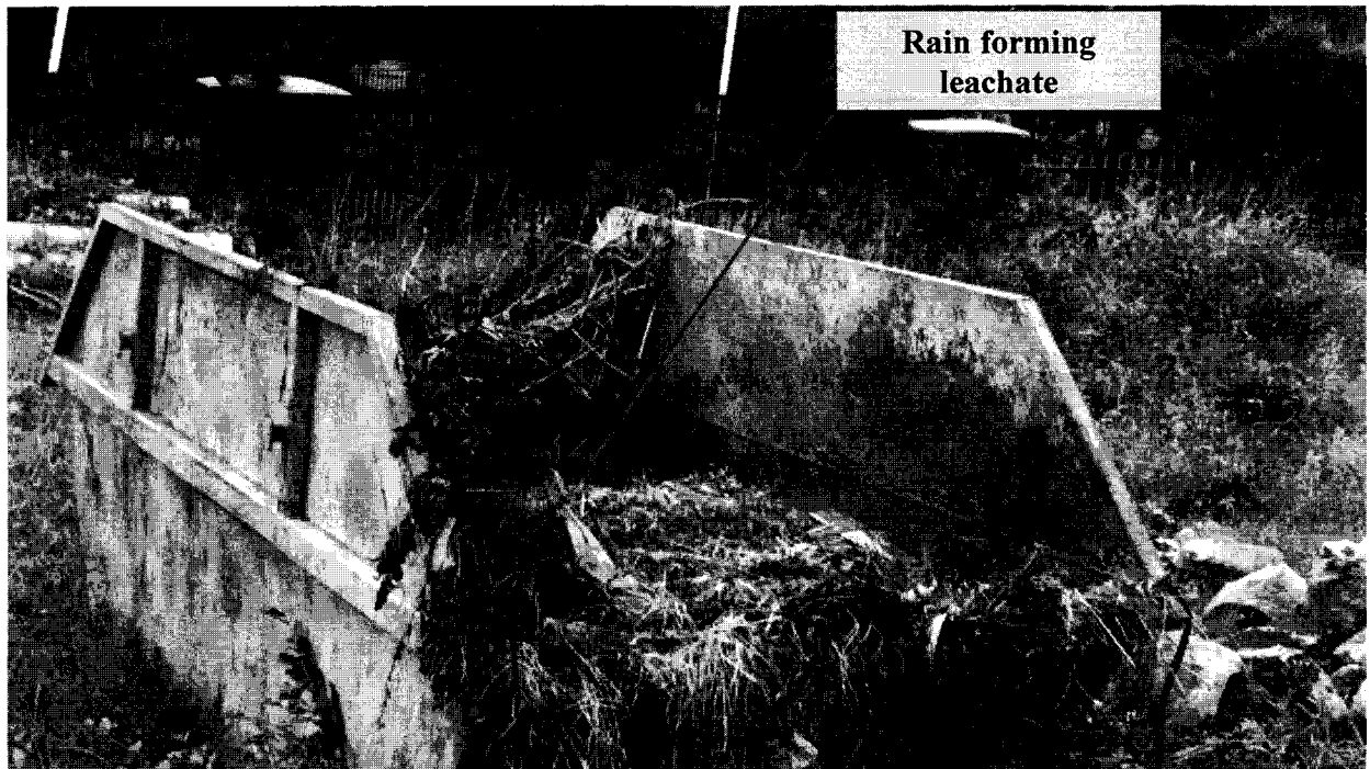
Figure 3-5: Solid Waste Skip filled with waste and leachate waiting to be emptied inside the municipal office
