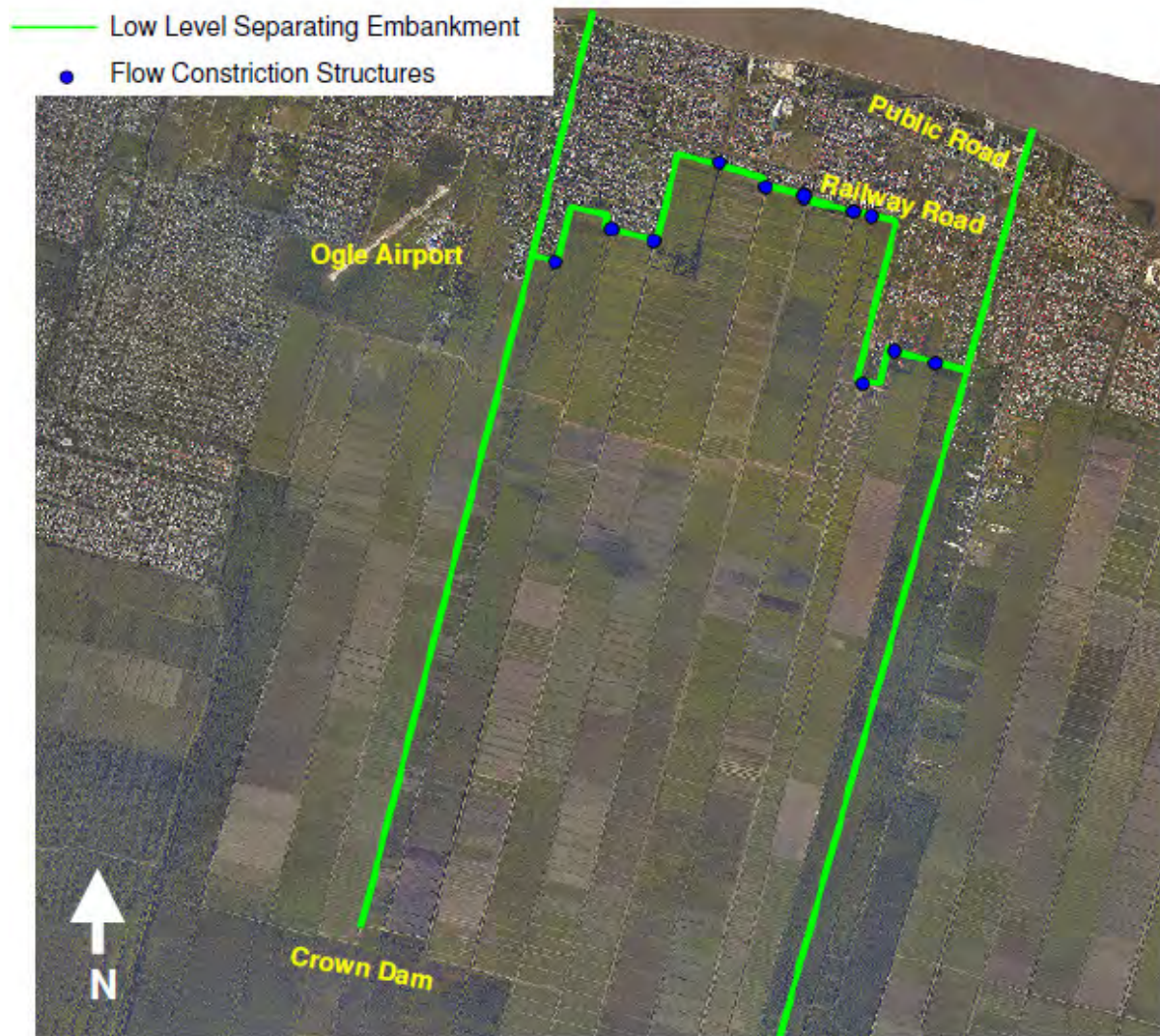
Figure 1.3: General Arrangement of Proposed Works at Montrose
