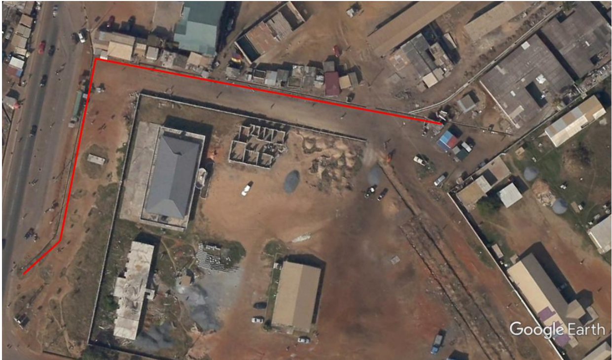
Red line showing the route where drains will be reconstructed at Naval Base area in Tema New Town
