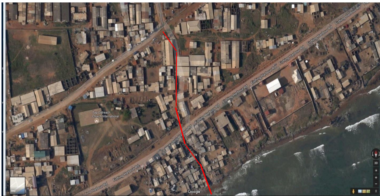
Red line showing the routes of the proposed drains construction in the Bankuman community in Tema Newtown
