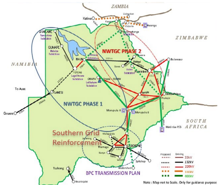
FIGURE 4.6 BOTSWANA'S TRANSMISSION GRID
