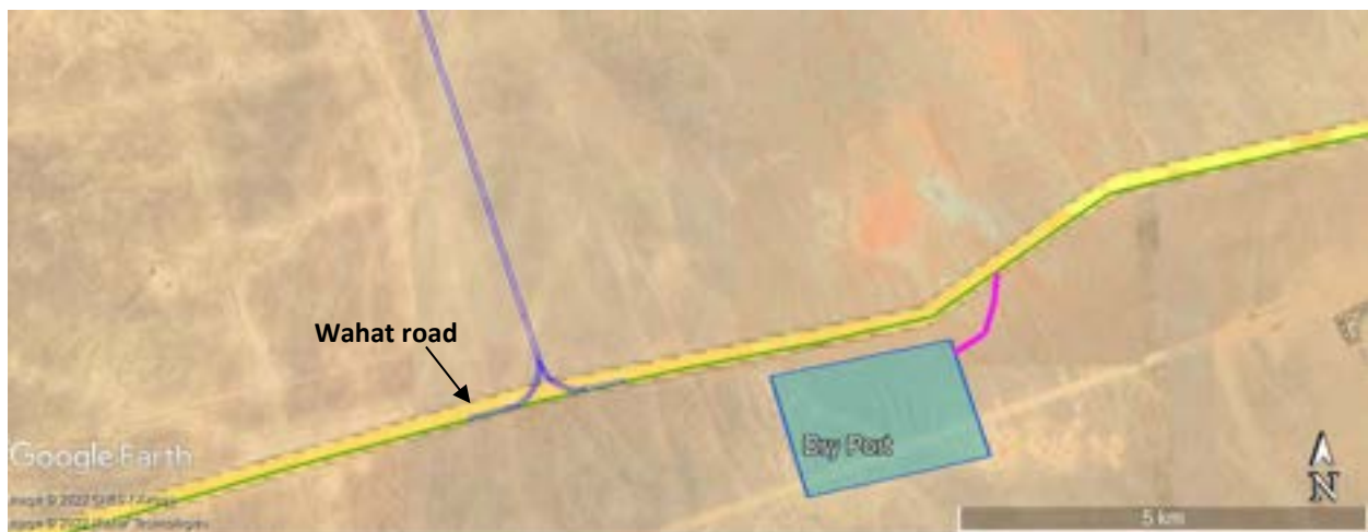
Figure 2-8: Intersection of the railway track with Wahat road, where there will be road flyover
