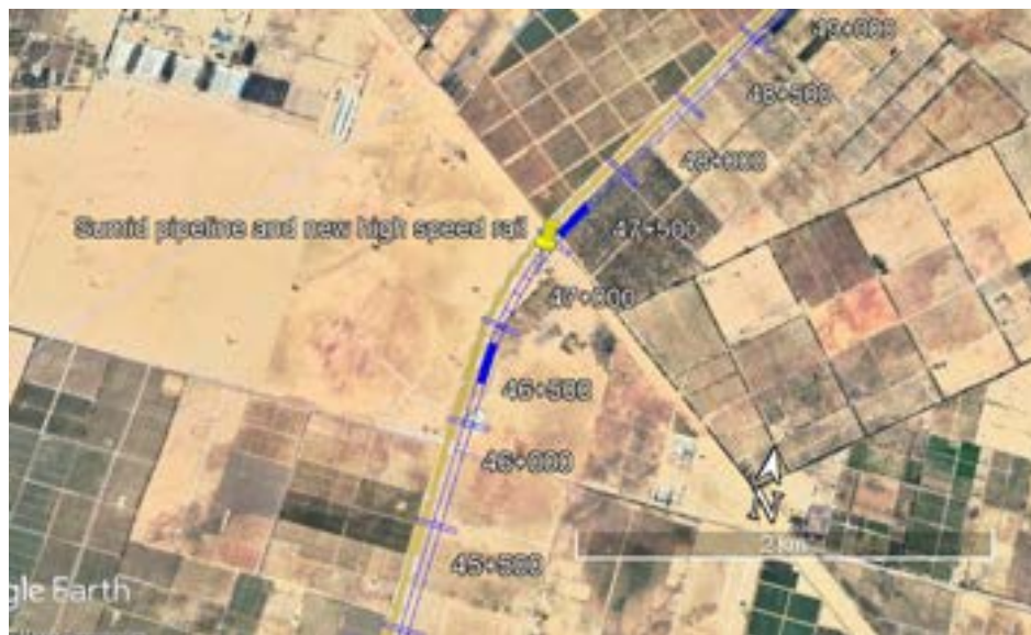
Figure 2-15: Intersection with Sumid pipeline and high-speed rail
