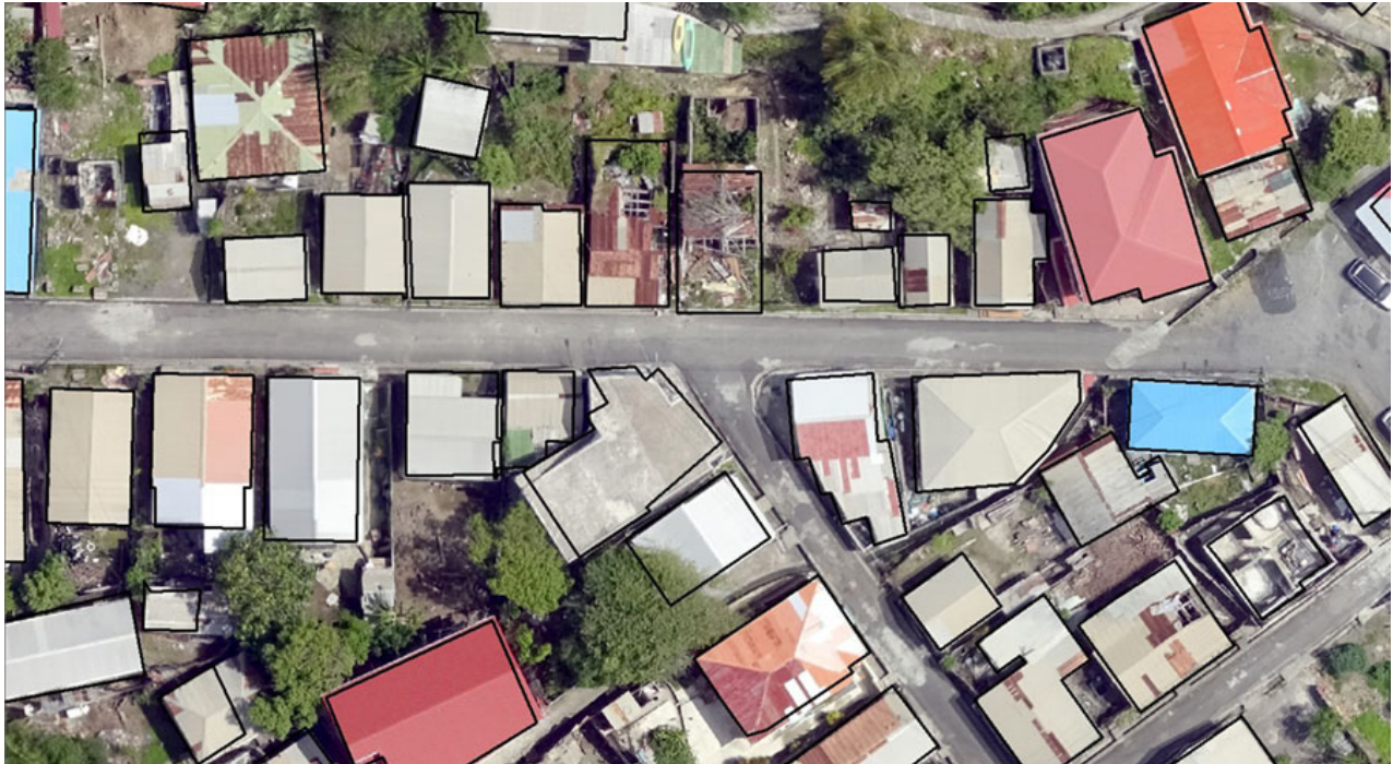
FIGURE 14: Delineated rooftop polygons overlaid on a drone-derived orthomosaic in St. Lucia
