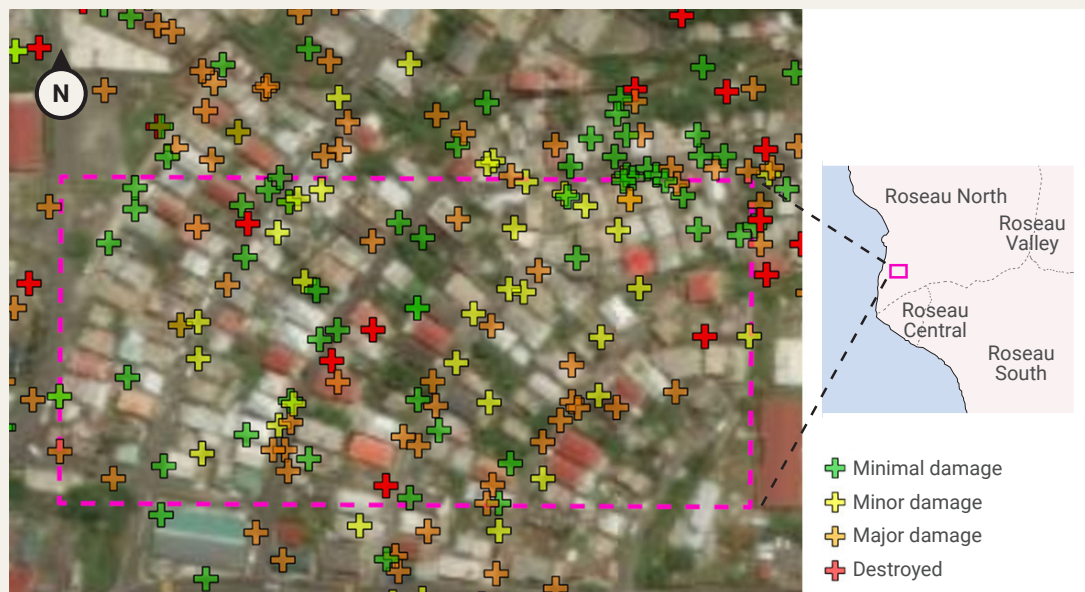
FIGURE PS-1: Housing data from a Dominica neighborhood overlaid on satellite imagery base map
