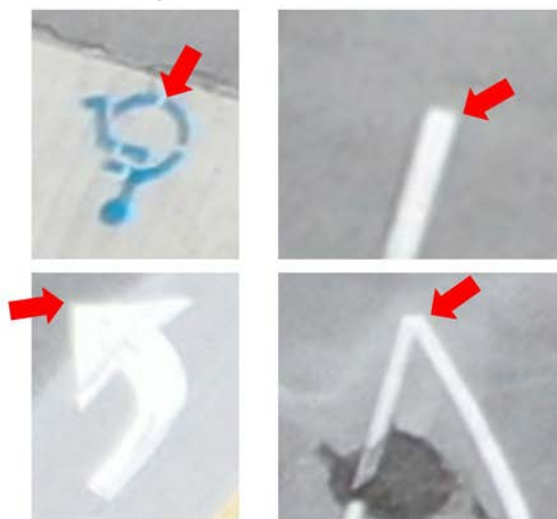
FIGURE 5: Examples of high-contrast ground control points for indirect georeferencing of drone imagery
