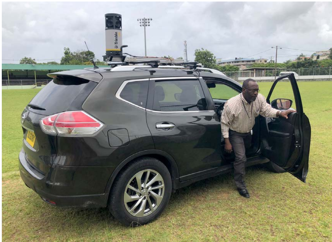
FIGURE 7: Trimble MX7 mobile mapping system used for street view data collection in St. Lucia
