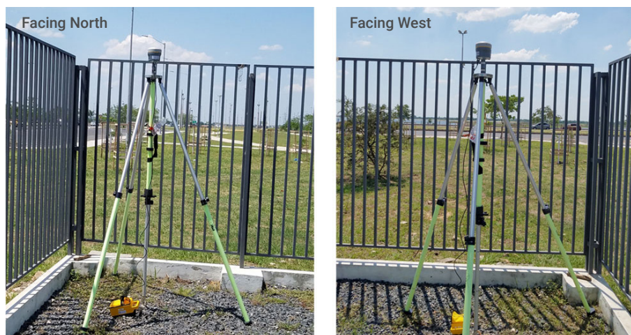
FIGURE 4: GNSS base station on a fixed-height tripod in a secure site with minimal overhead obstructions
