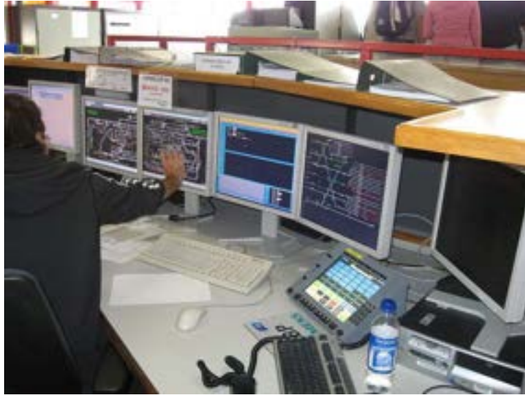
Figure 5-3 Electronic interlocking system
