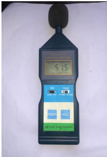
Noise Assessment – Noise Meter
