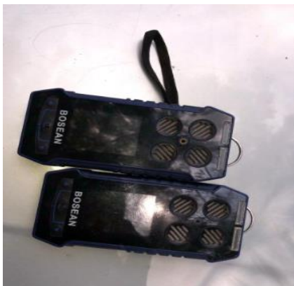
Air Quality Assessment - BH - 4S - Portable multi gas detector
