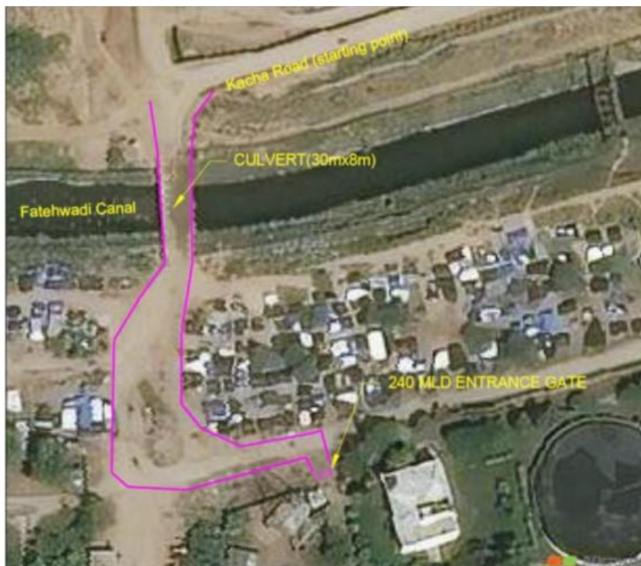
Figure 13 Present Status of Approach Road for 240 MLD STP and proposed road Repairs and upgradation
