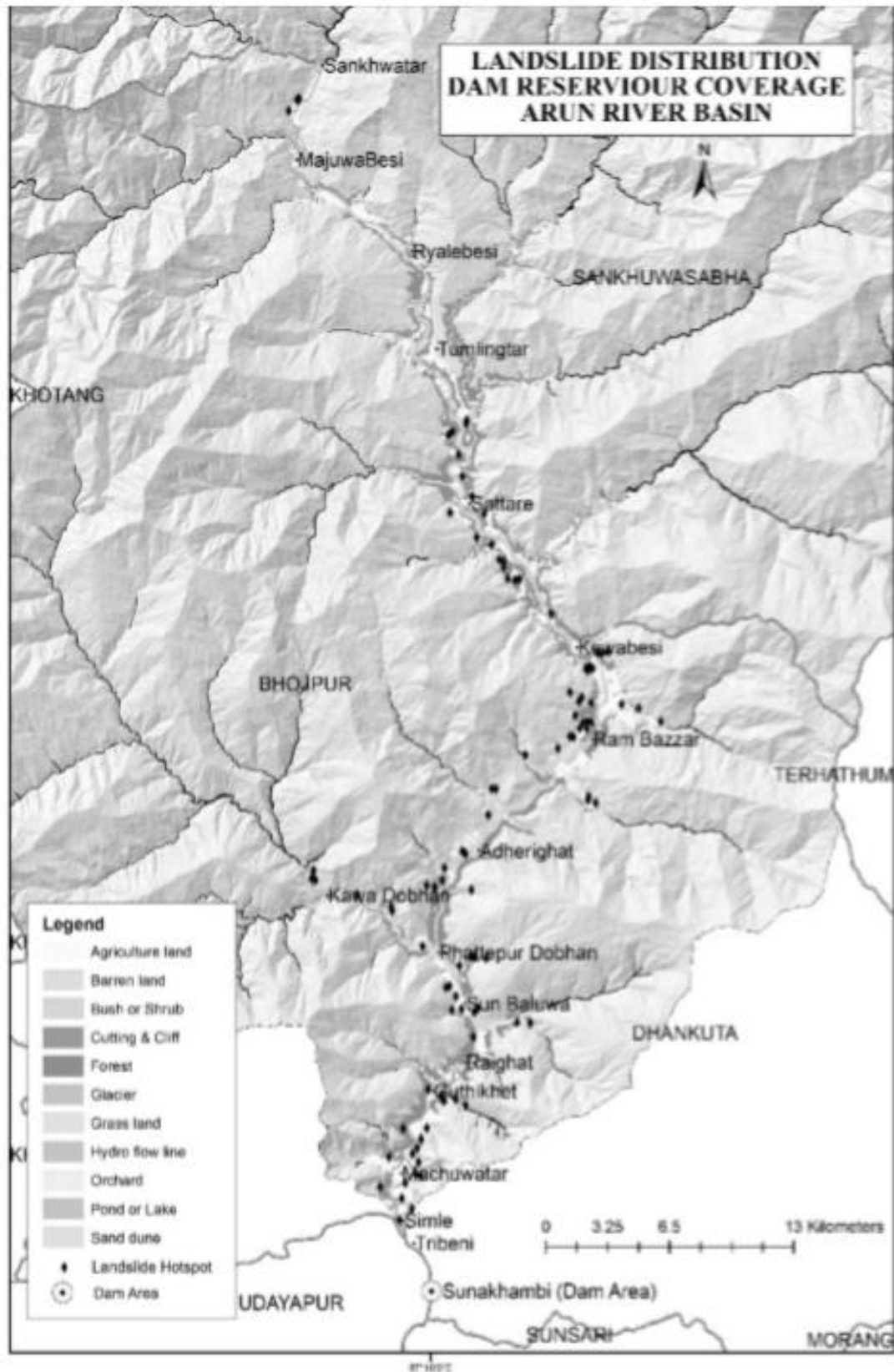
Figure 5.11: Landslide Hotspots in the Lower Arun Basin
