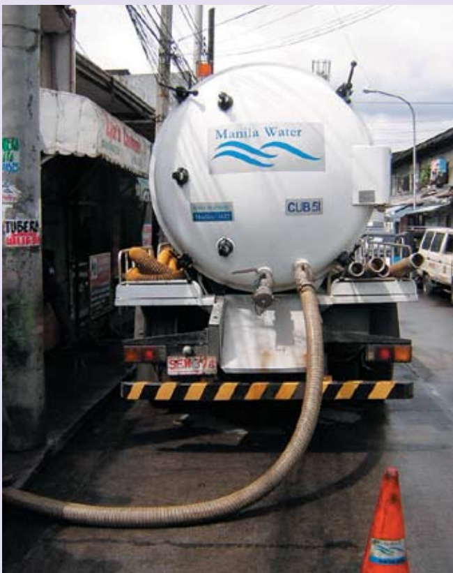
Regular desludging is undertaken in many parts of Manila. Source: Authors.
